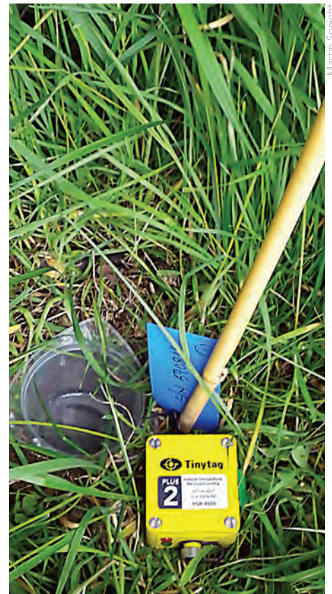
Pitfall trap and temperature/humidity data logger on a student project on insects in meadows, Oxfordshire
